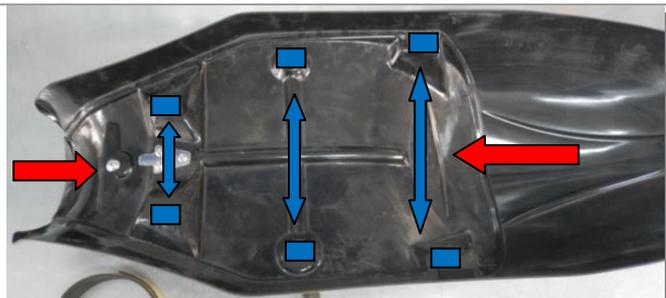
1. Place the seat cowl base upside down and screw the seat base with the cowl using the M6x15 bolts (**red arrows**).
