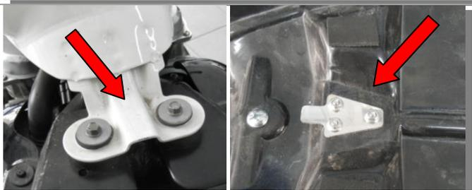
6. In order to fit the seat, front metal support must be placed in the same position as your old seat was fitted (pictures).
