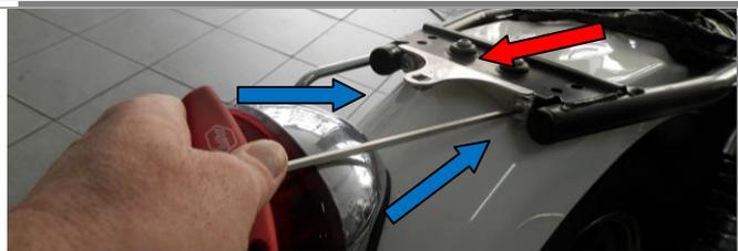
3. Fit the clip on metal support included in the package. The clip must be, as shown in the picture, with the square side downwards (**red arrow**). Screw metal support at the same position your old seat was fitted (using the original 2 x bolts from stage 2). Before tighten the bolts make sure it is parallel with the frame and on the higher spot (**blue arrows**).
