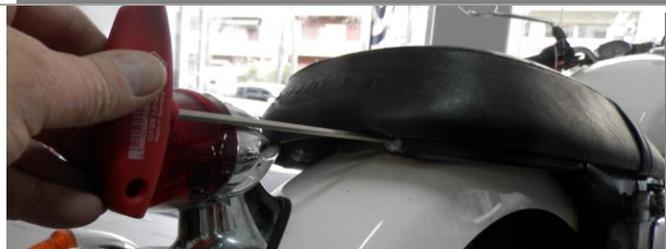
2. Remove the old seat and keep the 2 bolts. You will use them afterwards. Tool needed No 6 T shape allen-wrenche like the picture.
