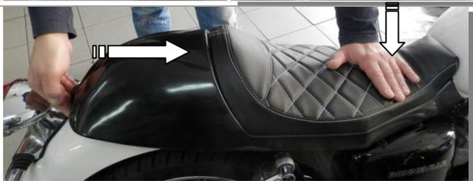
7. Place the seat as shown in the picture, putting pressure in the front part downwards in order to get in position and with your other hand move the seat forward. Make sure the seat is "locked" before moving to next stage. In the beginning fit is tight in order to avoid future gaps.
